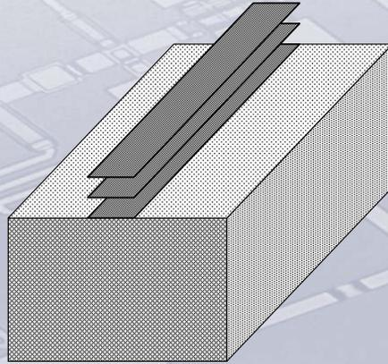
The Sonnet N-sheet model is shown here. Three sheets are shown in the figure. As we increase the number of sheets, and as the cell size becomes smaller and smaller, the answer should converge to the correct answer. Prior to version 9, we had to enter each sheet manually. For the 3-sheet model shown here, we would have three port 1's on this end and three port 2's on the other end.
