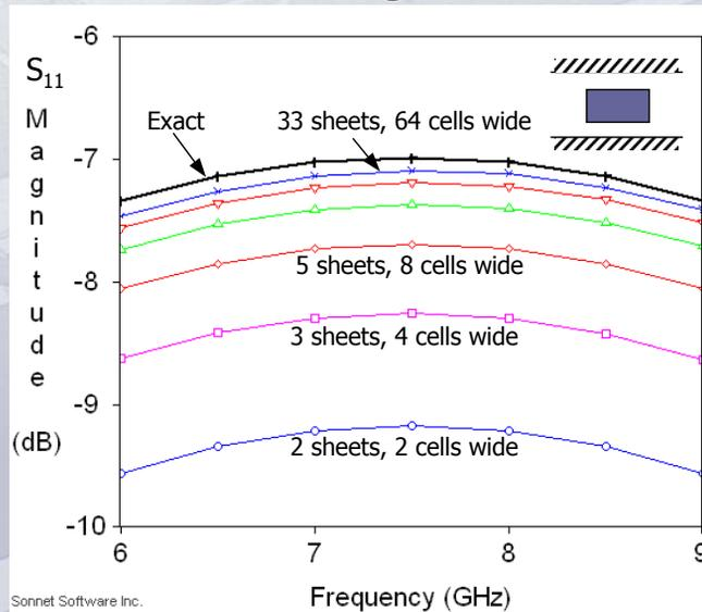
Circuit theory, using a  $Z_0$  of 30.8887 Ohms provides the curve labeled “Exact”. Here we can see how the  $S_{11}$  for a 10 mm long line converges as we increase the number of sheets and decrease the cell width (increase the number of cells across the width of the line).
