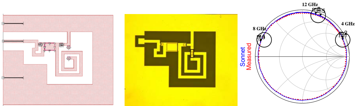
Figure 4 – Sonnet Simulations vs. measured s-parameter result from the resonator (1 – 14 GHz)
