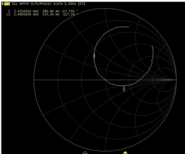
Figure 3: Measured element return loss.
