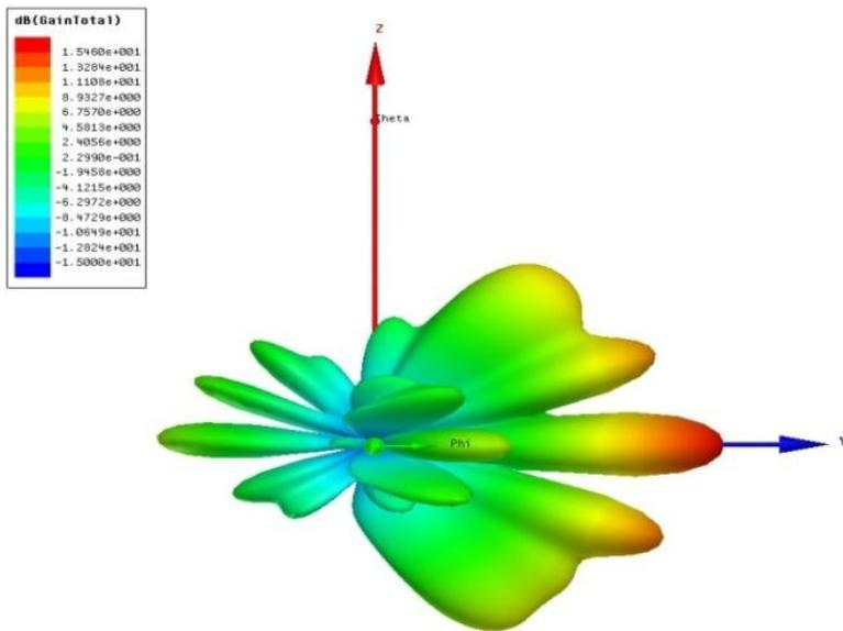
Figure 4: Antenna Pattern without phase shifts.
