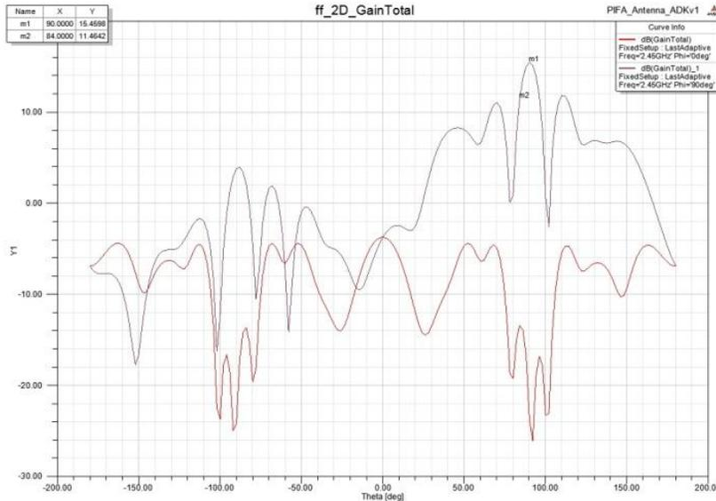
Figure 5: Antenna Pattern without phase shifts.
