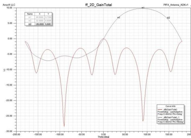
Figure 1: Element Gain Pattern
