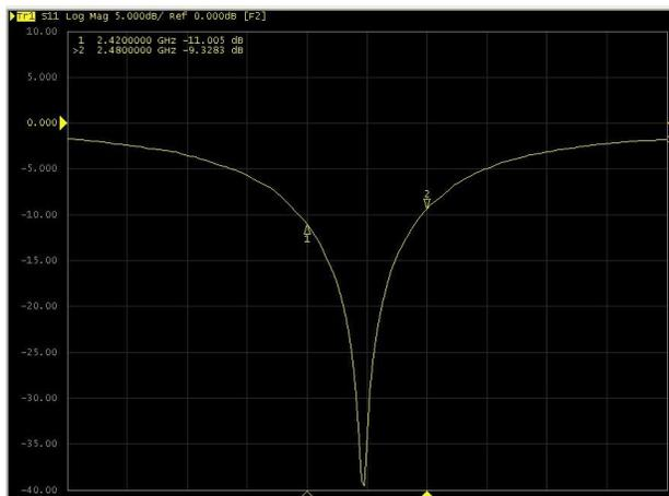
Figure 2: Measured element return loss.
