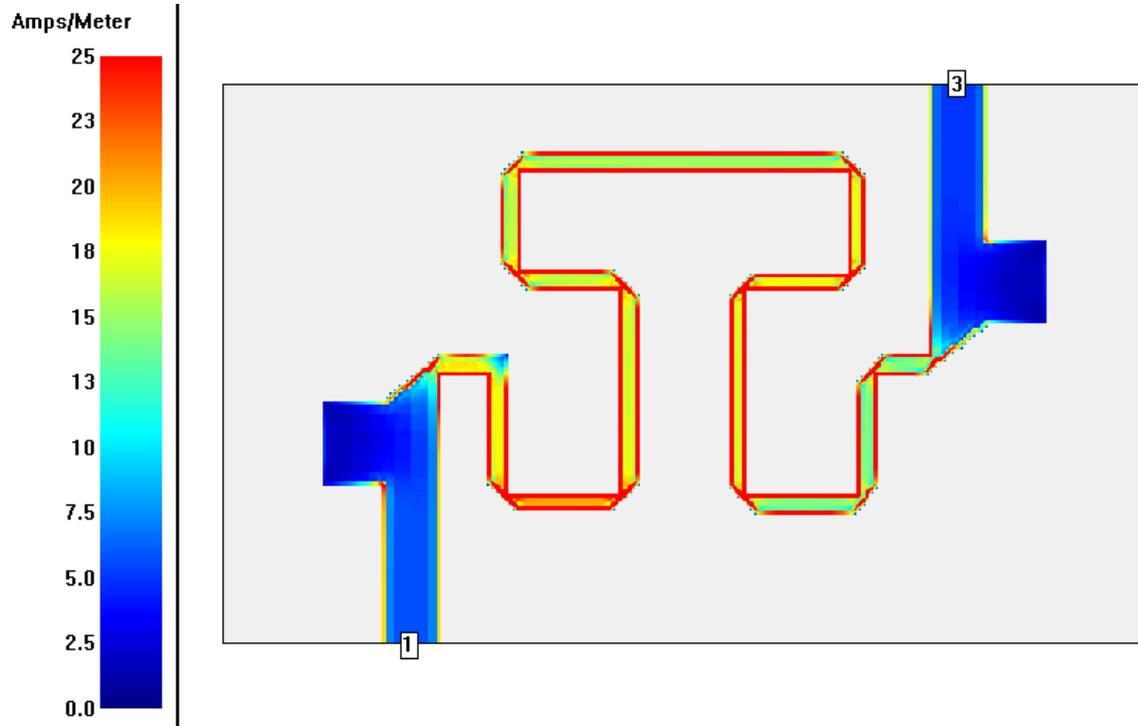
Fig. 8. Current distribution on the coupler (port1 and port3).
