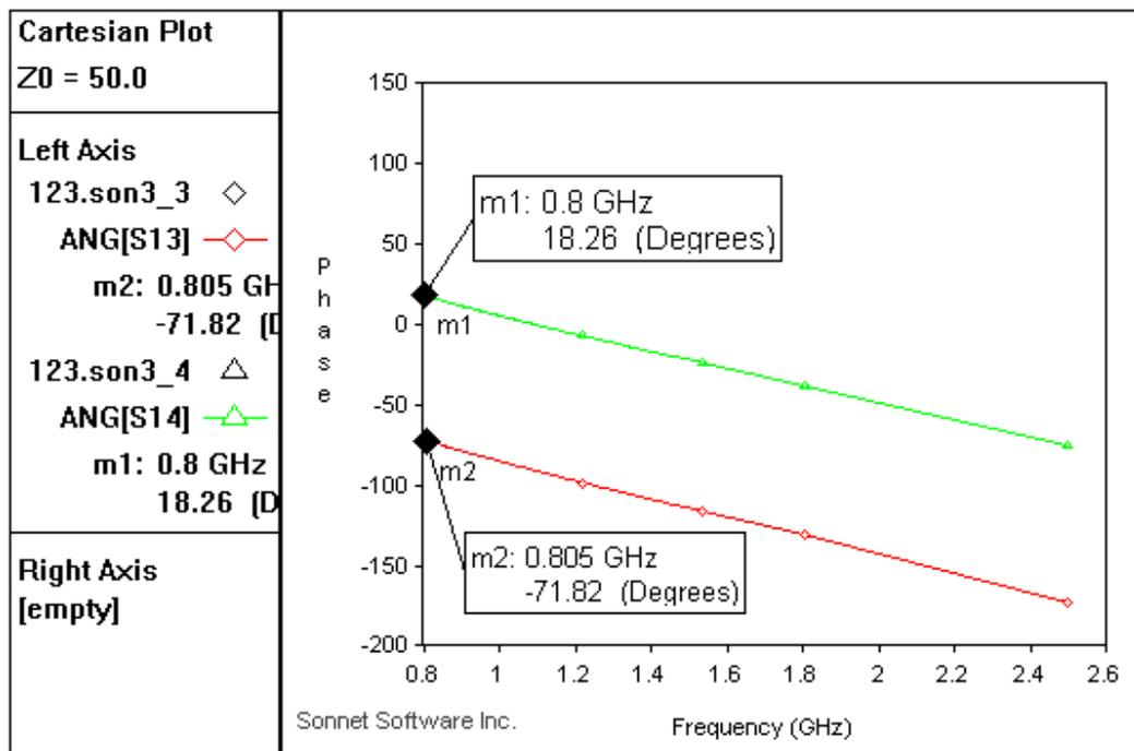
Fig. 7. Phase difference between the coupled and thru port.
