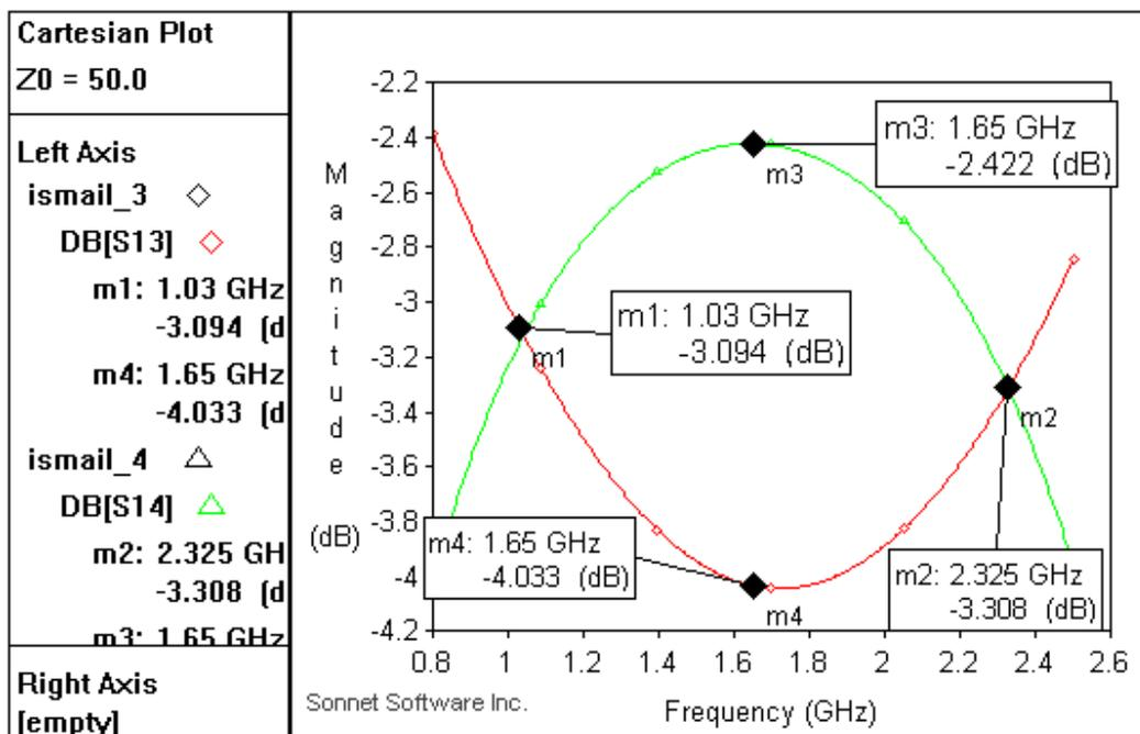
Fig. 5. Amplitude Balance.
