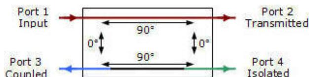
Fig.1. 3dB Hybrid multiplexer.
