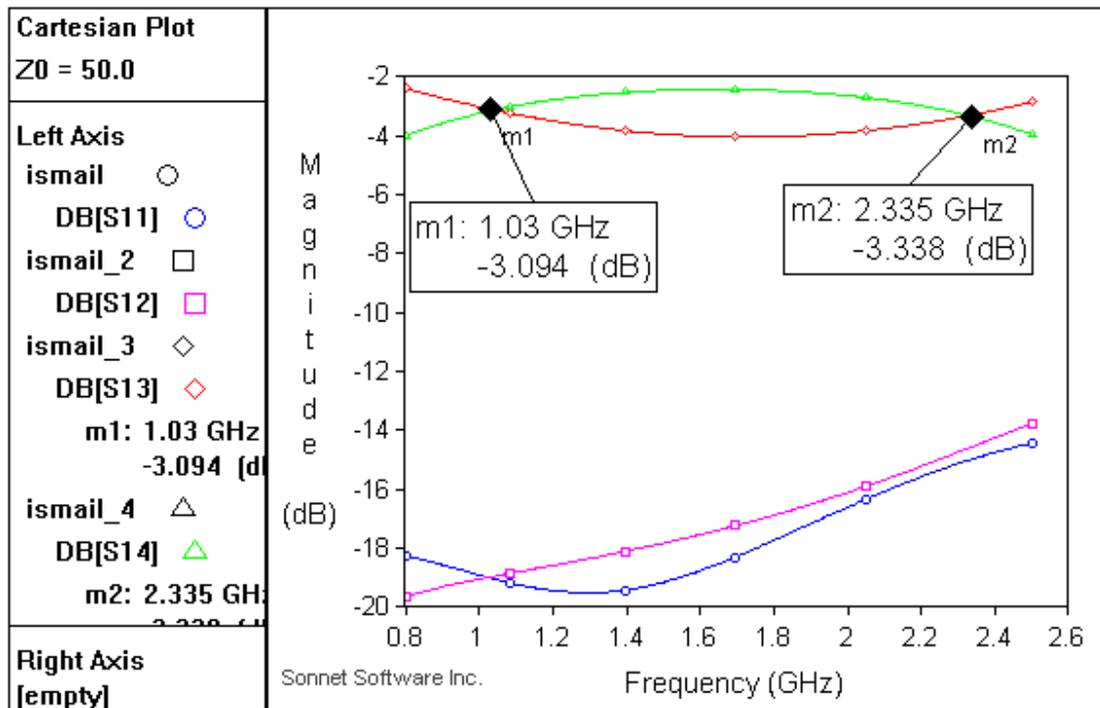
Fig. 4. S-parameters of the Coupler.
