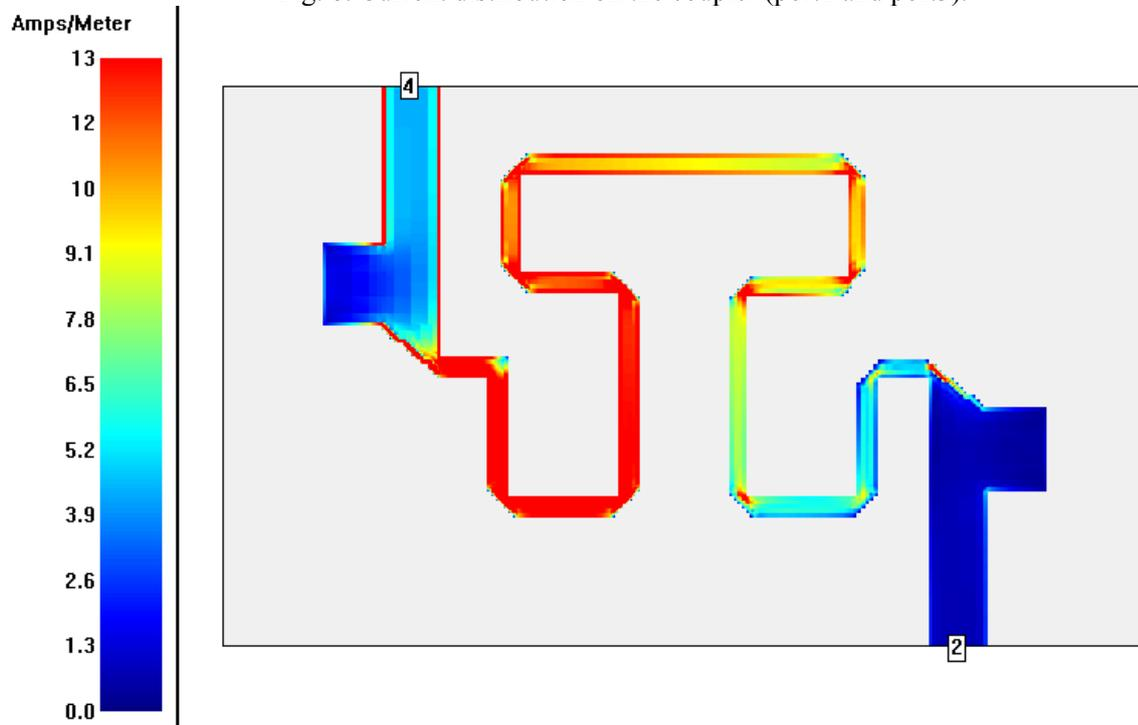
Fig. 9. Current distribution on the coupler (port2 and port4),
