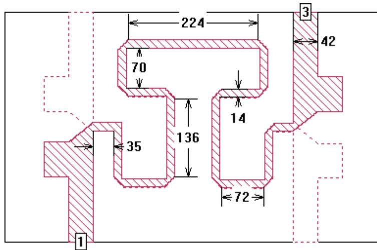
Fig. 2. Top view and dimensions of the coupler (mils).
