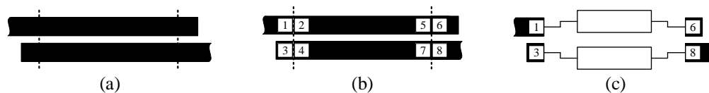
Fig. 5. Illustration of TSM with embedded tuning elements: (a) a coupled microstrip line of length L , (b) coupled line with co-calibrated ports inserted, (c) tuning model of the coupled line: middle section is replaced by the microstrip model (tuning element).
