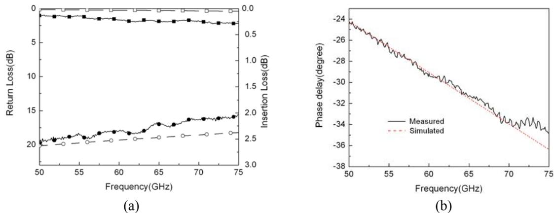
Fig. 8. Measured and Simulated (a) S-parameter performance and (b) phase delay of the  $36^\circ$  CPW bend.
