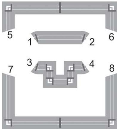
Fig. 5 The phase shifter delay line topology.
