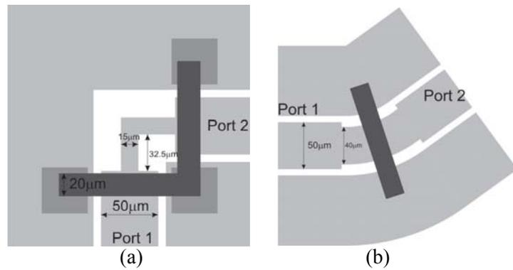
Fig. 6. Layout of the (a) 90° and (b) 36° bend.
