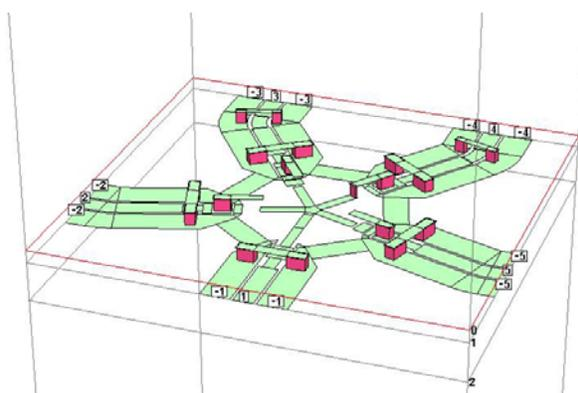
Fig. 2. The 3D SONNET representation of the SP4T RF-MEMS switch.
