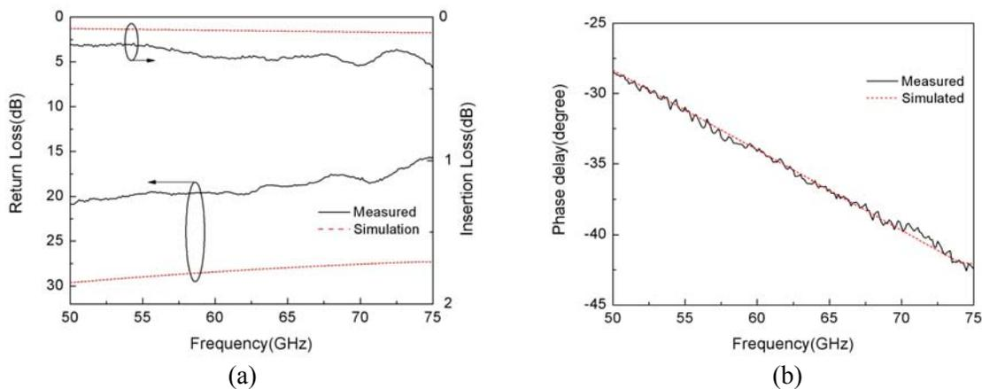
Fig. 7. Measured and Simulated (a) S-parameter performance and (b) phase delay of the 90° CPW bend.
