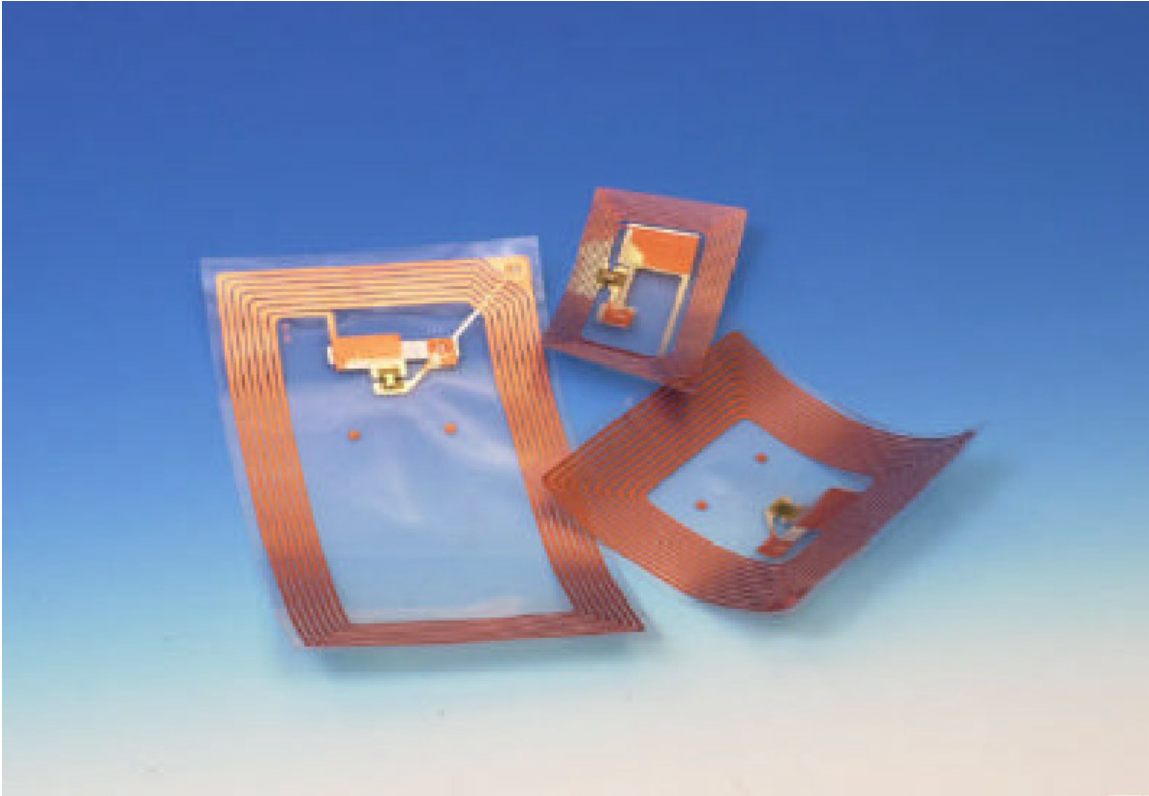
Figure 1. Texas Instruments' "Tag-It" can be laminated into tags, cards, etc.
