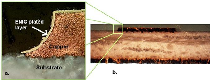
Fig. 1. A cross section of a microstrip line plated with an ENIG process. The nickel-phosphorous plating is visibly conformal. The gold coating is generally too thin to be visible [3].
