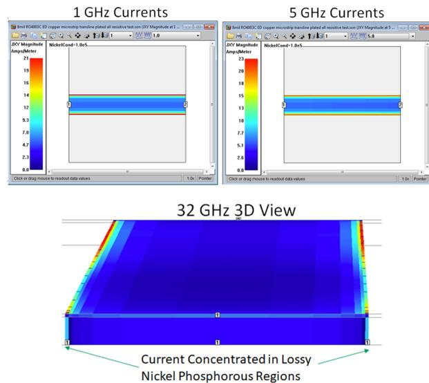
Fig. 3. Simulated cross-sections from Sonnet at 1 GHz (top left), 5 GHz (top right) and 32 GHz (bottom). With increasing frequency, the current is increasingly in the sides of the conductor, where the more-lossy nickel-phosphorous resides.
