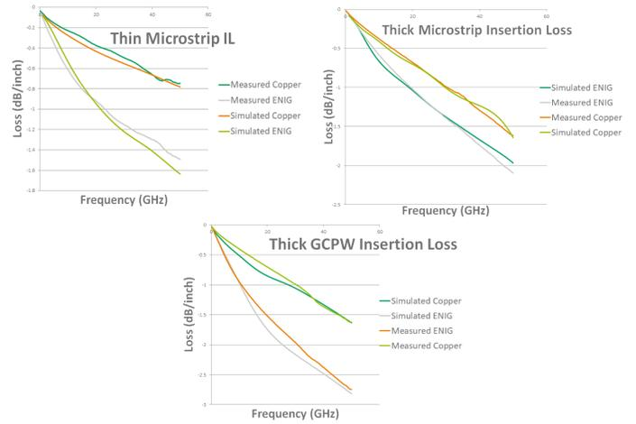
Fig. 4. Simulated vs measured data for the thin microstrip test (top left), thick microstrip test (top right) and thick GCPW test (bottom). Agreement is reasonable and the frequency behavior of the ENIG plating suggests strong dependence on edge-effect.
