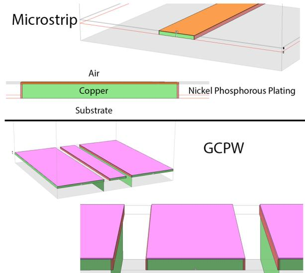
Fig. 2. Models in Sonnet including the nickel-phosphorous plating as being conformal on exposed surfaces of the main copper conductor. The sidewalls are composed of thick metal with the conductivity of nickel-phosphorous. Microstrip (Top) and GCPW (Bottom) are pictured.
