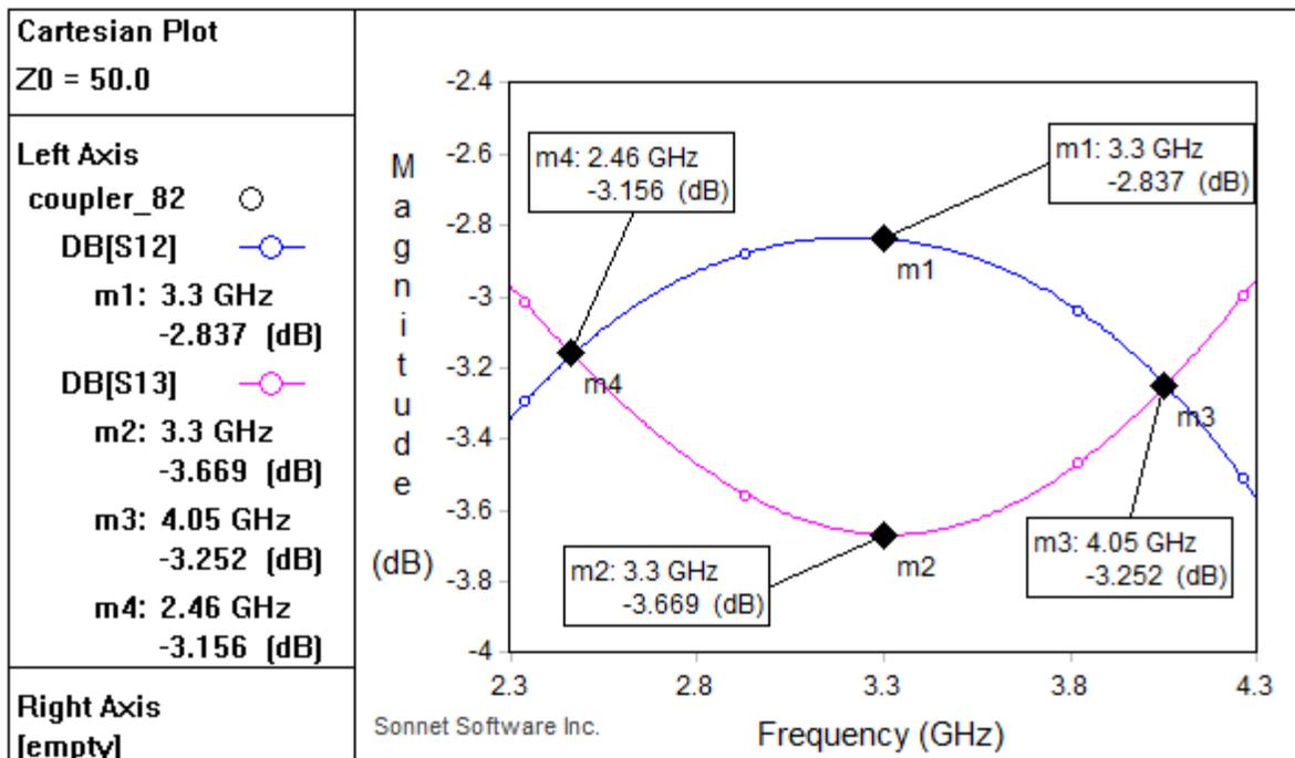
Fig. 4. A close-up view to show the Amplitude Balance.
