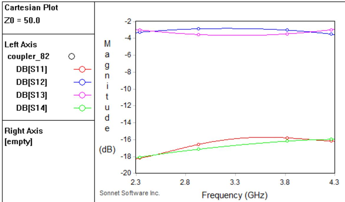
Fig. 3. S-parameters of the Coupler.
