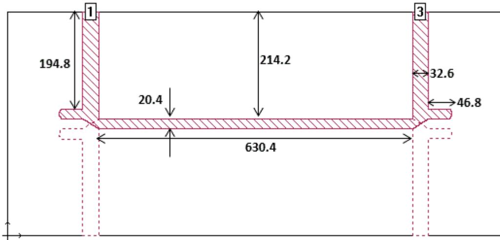
Fig. 1. Top view and dimensions of the coupler (mils).
