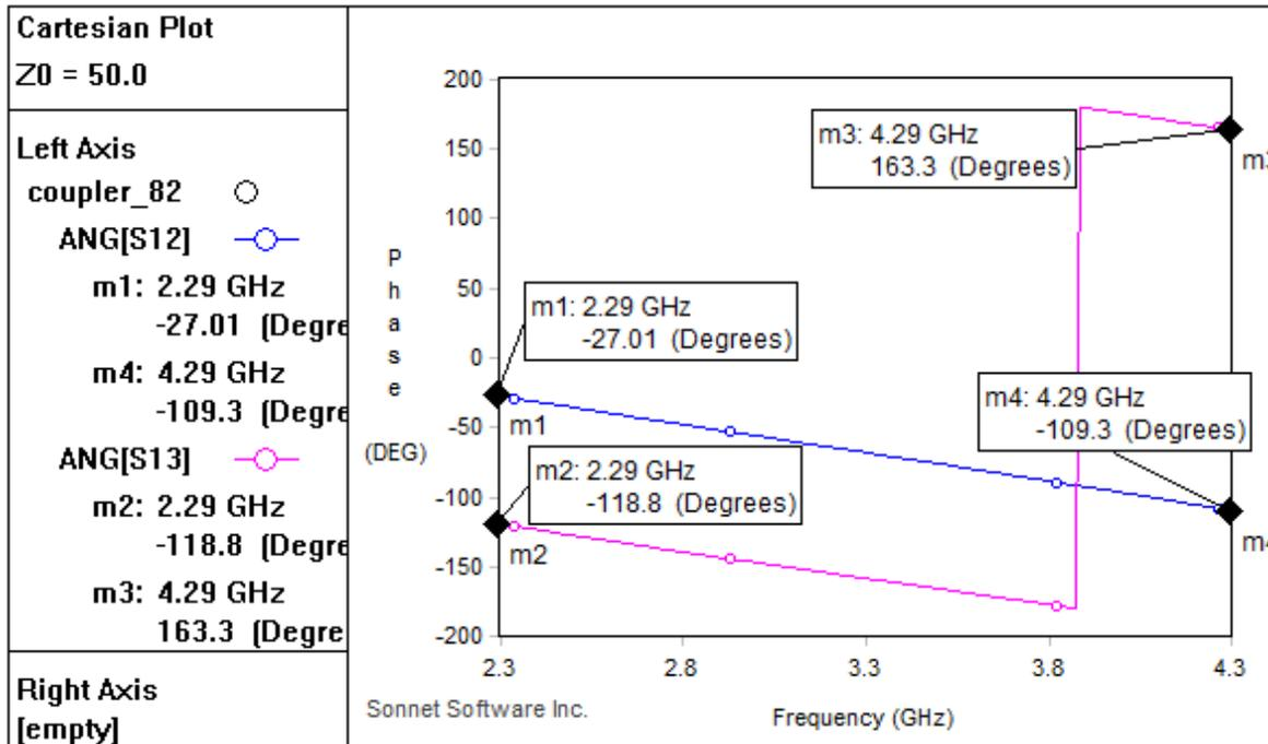
Fig. 5. Phase difference between the coupled and thru port.
