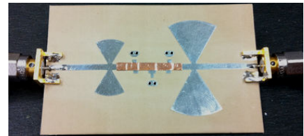
Fig. 3d. Band reject test board.
