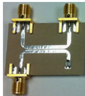
Fig. 3c. Directional coupler test board.
