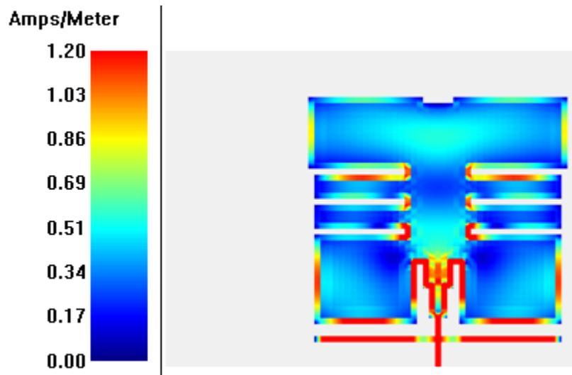
Fig. 5. Current distribution on the antenna at 7.1 GHz.
