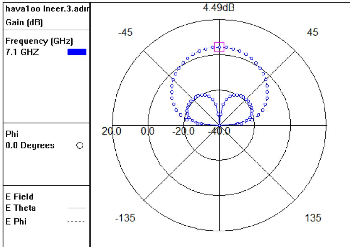
Fig. 4. Far field radiation pattern of the antenna at 7.1 GHz.
