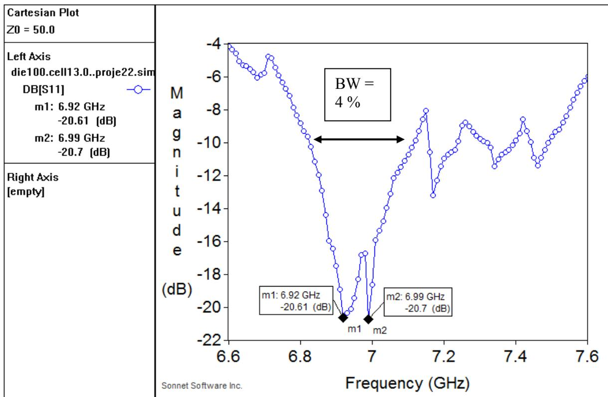
Fig. 8. Return loss of the patch antenna.
