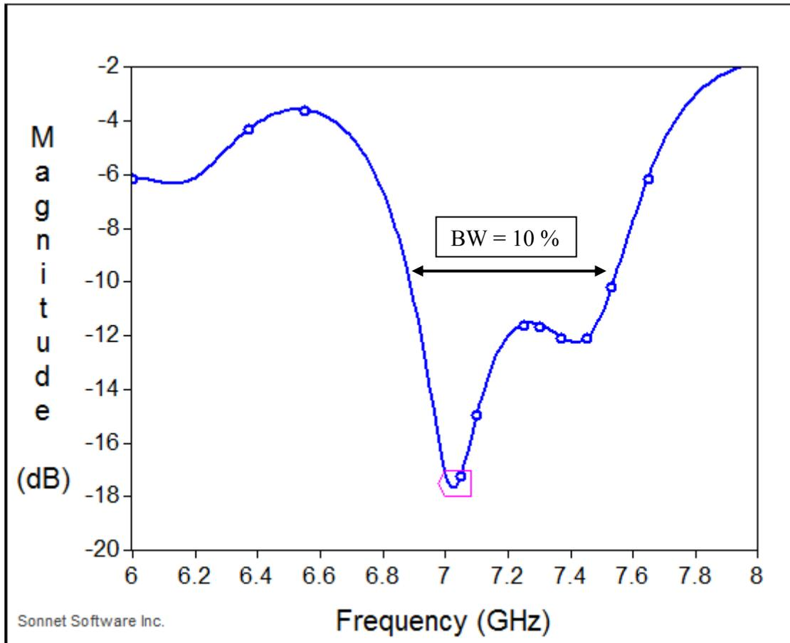
Fig. 3. Return loss of the patch antenna.
