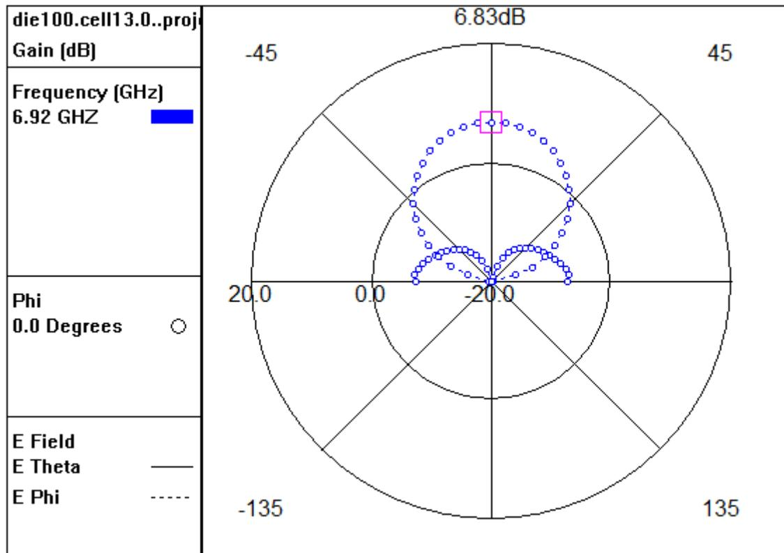
Fig. 9. Far field radiation pattern of the antenna at 6.92 GHz.
