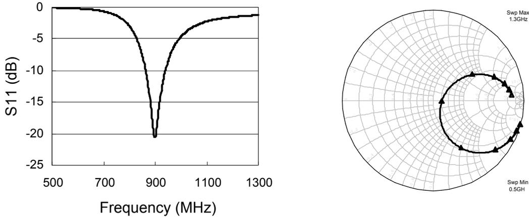
Fig. 2. Simulated  $S_{11}$  and impedance of regular half-wavelength dipole on a 0.4mm FR-4 substrate ( $\epsilon_r = 4.2$ ).
