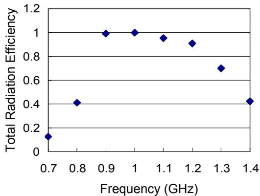
Fig. 7 Total efficiency versus frequency of the quasi log-periodic antenna
