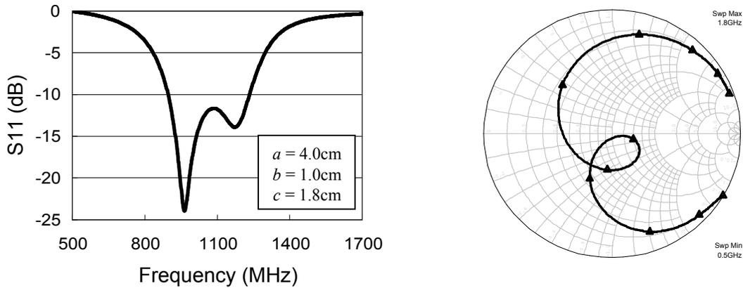
Fig.3. Simulated  $S_{11}$  and impedance of the quasi log-periodic antenna on a 0.4mm FR-4 substrate ( $\epsilon_r = 4.2$ ).
