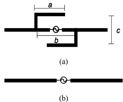
Fig. 1. (a) Structure of the proposed quasi log-periodic antenna and (b) Structure of the conventional half-wavelength dipole.
