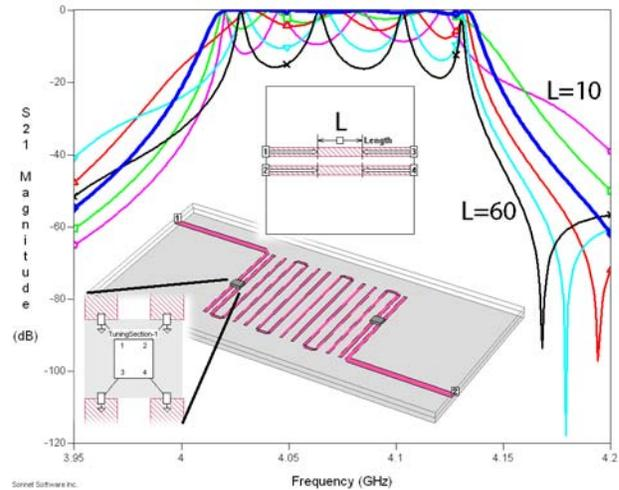
Fig. 3. The six resonator hairpin filter has two sets of perfectly calibrated ports (one set detailed, lower left) placed in the input and output coupled sections. A length,  $L$ , of coupled line (central inset) is inserted into each set of ports. As  $L$  is varied from 10 to 60 mils, step of 10 mils, new results are instantly available. The thick blue line ( $L=30$ ) corresponds to the filter of Fig. 2. Notice the over 100 dB dynamic range.
