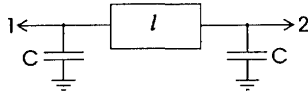
Figure 3. The equivalent circuit theory model of a length, l , of transmission line includes a port discontinuity at each end of an ideal TEM transmission line.
