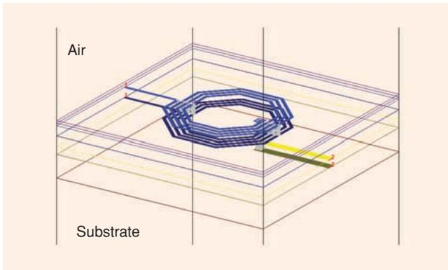
**Figure 3.** 3-D view of the two-sheet per thick metal layer model of the 3.3-nH inductor.
