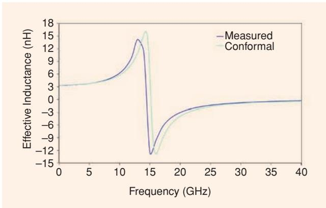
**Figure 4.** Measured effective inductance compared to conformal mesh simulations of the inductor.
