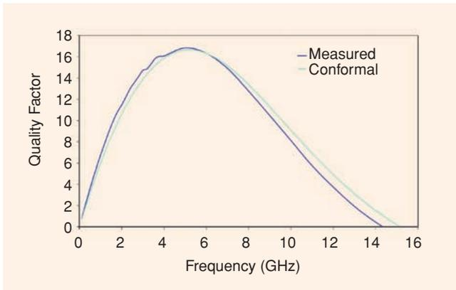
**Figure 5.** Measured  $Q$  factor compared to conformal mesh simulations of the inductor.
