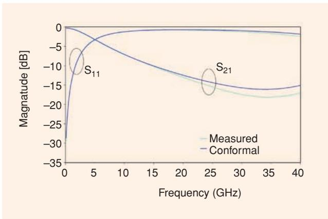
**Figure 6.** Plots of the magnitude of  $S_{11}$  and  $S_{21}$  obtained from measurement and from conformal mesh simulation.
