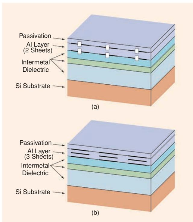
**Figure 2.** CPW cross-section for the 4- $\mu\text{m}$  aluminum layer. (a) Two metal sheet base case. (b) Three metal sheet case.
