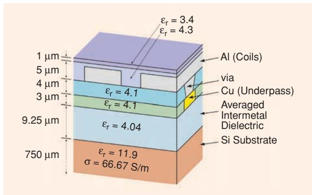
**Figure 1.** IBM CMRF8SF high-Q factor inductor cross-section with the weighted average dielectric constants and layer thicknesses used in the simulator.
