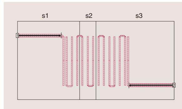
**Figure 3.** Partitioning a filter between coupled resonators results in failure of the topological partitioning because coupling between partitioned sections is not included. Partitioning between the legs of a hairpin resonator might result in decreased accuracy because coupling between the legs is not included.
