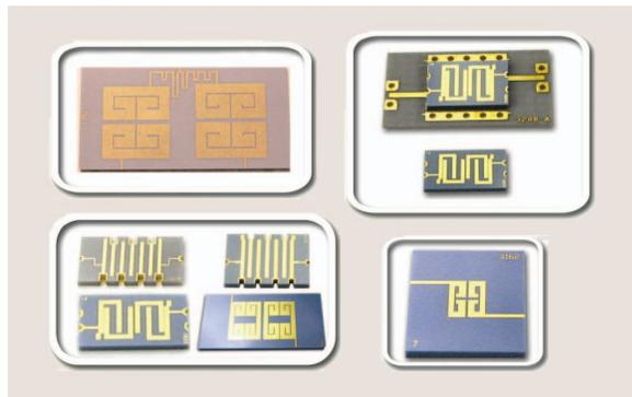
**Figure 1.** Filters on ceramic designed by Dielectric Laboratories are the results of new microwave design methodologies that use numerous additional ports to facilitate rapid design closure.
