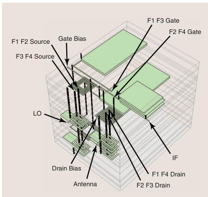
**Figure 12.** The transmitter portion of a module analyzed with EM analysis based topological partitioning driving artificial neural network model generation. The complete circuit includes a 3-D aspect requiring use of multiple EM tools.
