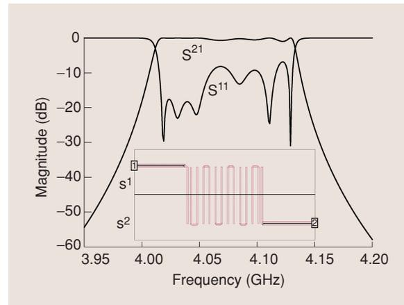
**Figure 2.** Divide and conquer, or topological partitioning, applied to a filter. Split, as indicated, in half, each half EM analyzed and connected back together using circuit theory yields results exactly identical to the EM analysis of the complete filter (from [9]).
