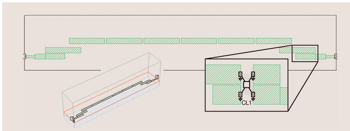
**Figure 8.** Bandpass filter from Dielectric Laboratories illustrating the principle of tuning ports (in the inset at right) for the output section of the filter. When a full set of tuning ports are in place, filter tuning and modifications proceed at circuit theory speed.
