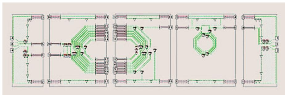
**Figure 4.** A circuit on silicon from NXP is partitioned into five small circuits. Each small circuit is EM analyzed and connected back together using circuit theory yielding results almost identical an EM analysis of the complete circuit (from [12]).
