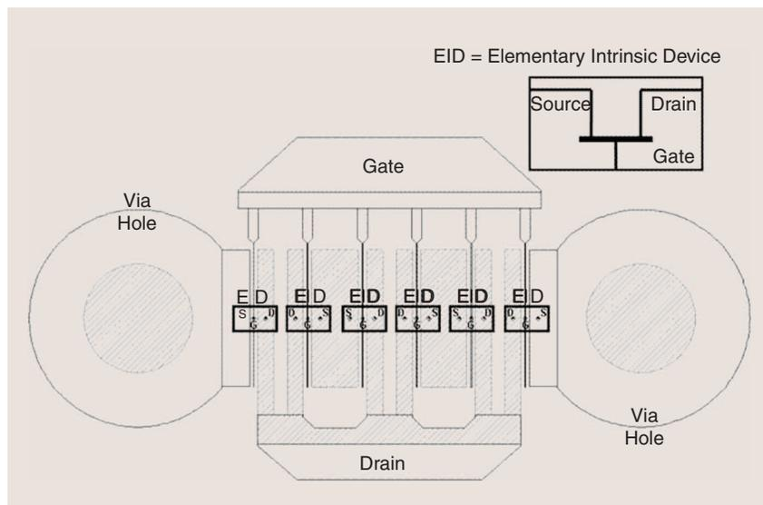
**Figure 6.** Functional partitioning applied to a power FET allows the passive parasitics of the FET to be evaluated by EM analysis with internal ports on each FET finger allowing connection of the nonlinear sources and bias-dependent passives. This model is easily scaled (from [13]).
