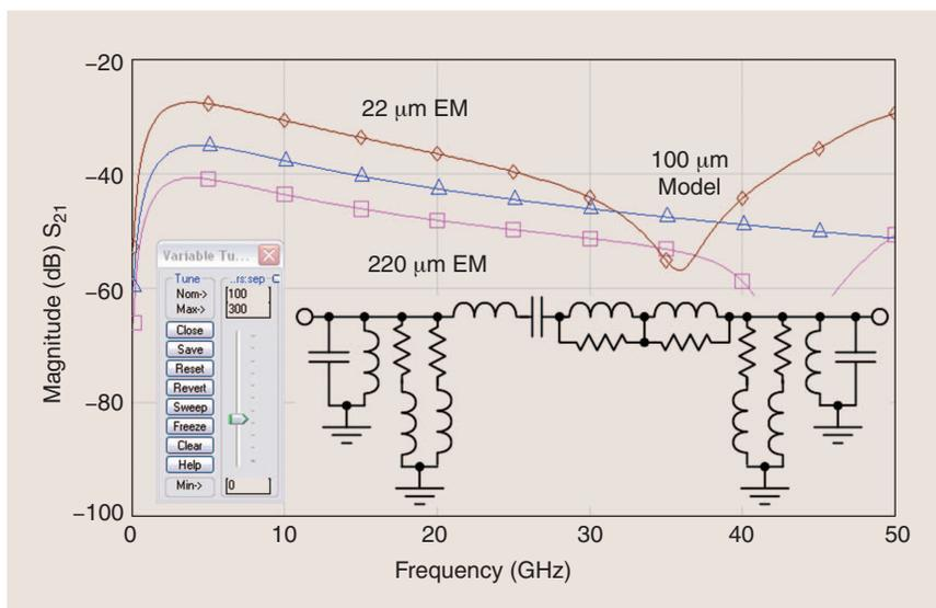
**Figure 11.** The synthesized lumped model for the coupled inductors of Figure 10. Each RLC is a simple function (linear up to cubic) of the inductor separation. The model is evaluated for an inductor separation of 100  $\mu\text{m}$ , midway between the EM results shown for 22  $\mu\text{m}$  and 220  $\mu\text{m}$  separation; after [12].
