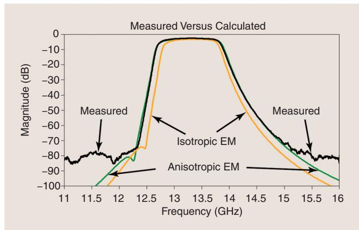
**Figure 9.** Typical measured versus calculated for the filter of Figure 8 indicates that including the anisotropy of the substrate in the EM analysis is critical for success on first fabrication. The “isotropic” analysis uses a dielectric constant “tuned” to give the correct center frequency, yielding unacceptable results.
