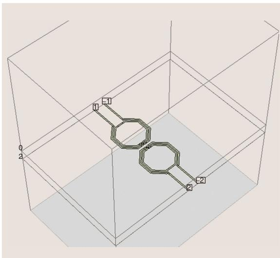
**Figure 10.** Two mutually coupled spiral inductors on silicon are modeled as a function of their separation (the gap between the two inductors), after [12].
