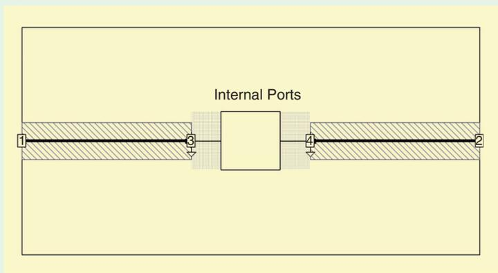
**Figure S1.** A simple circuit provides an acid test for internal ports. When there are hundreds of internal ports, even small port calibration error is magnified.
