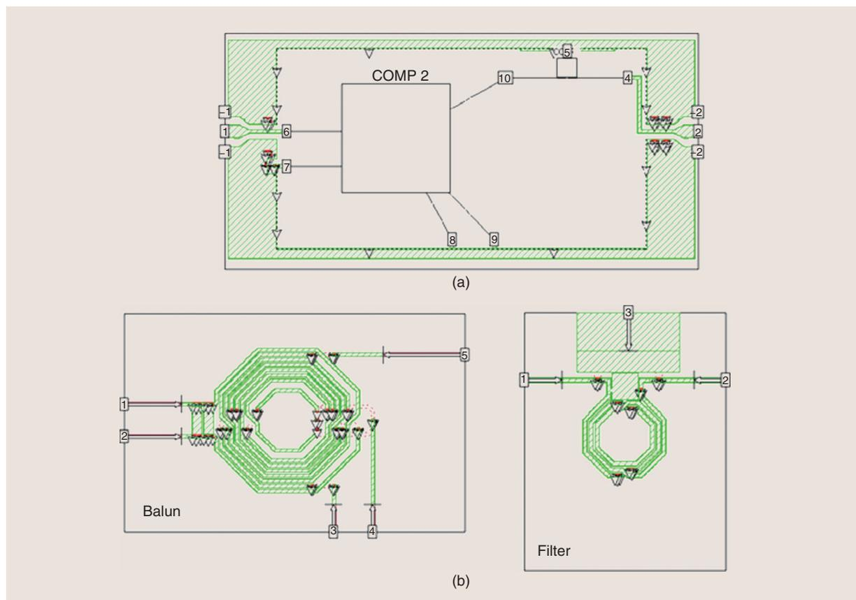
**Figure 5.** Functional partitioning separates (a) a circuit based on function with internal ports added for (b) each component that is analyzed separately (from [12]).
