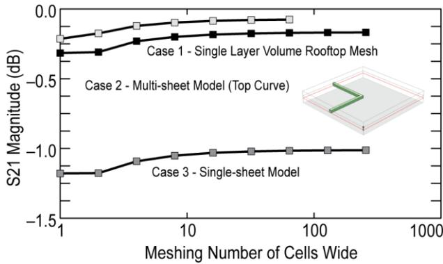
Fig. 2. Convergence analysis of a thick stripline with square cross-section. Case 1 uses a single layer of volume rooftop subsections. Case 2 (top curve) uses multiple infinitely thin sheets of current. Case 3 uses a single infinitely thin sheet of current. Results are plotted as cell size is reduced.
