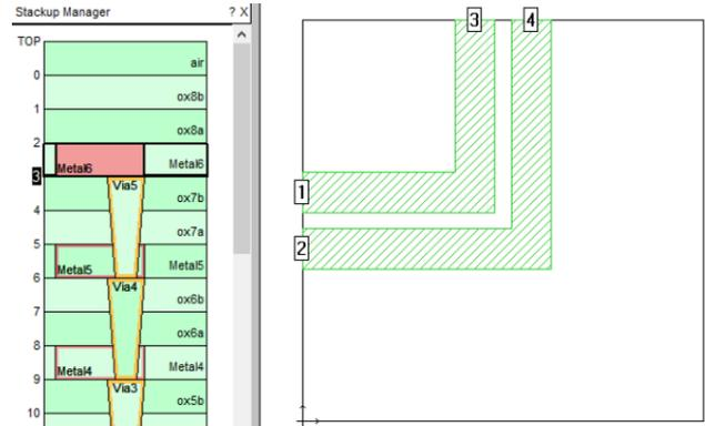
Fig. 3. Stackup and layout for the extremely thick coupled line validation test. A generic stackup is modified by changing Metal 6 to a thickness of 30  $\mu\text{m}$ . The line widths are 6  $\mu\text{m}$  and the line gap is 2.4  $\mu\text{m}$ . Results and 3-D view of the circuit in Fig. 4..
