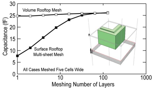
Fig. 4. The volume rooftop subsections provide a nearly converged answer for the interline capacitance even with only one layer. The multi-sheet surface rooftop model requires 33 sheets to realize a similar reduction in error.
