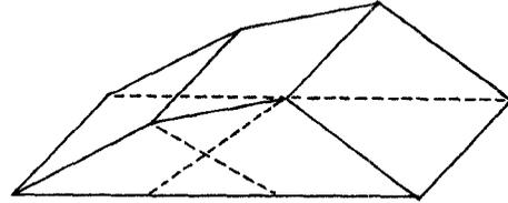
Fig. 3. Two rooftop functions placed on overlapping rectangles give a piecewise linear approximation to the current in the direction of current flow. Additional rooftop functions placed side by side will provide a step approximation to the surface current in the direction lateral to current flow.
