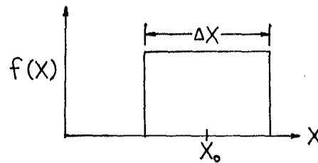
Fig. 4. The rectangular pulse function is used to represent the current density on a subsection in the direction lateral to current flow.
