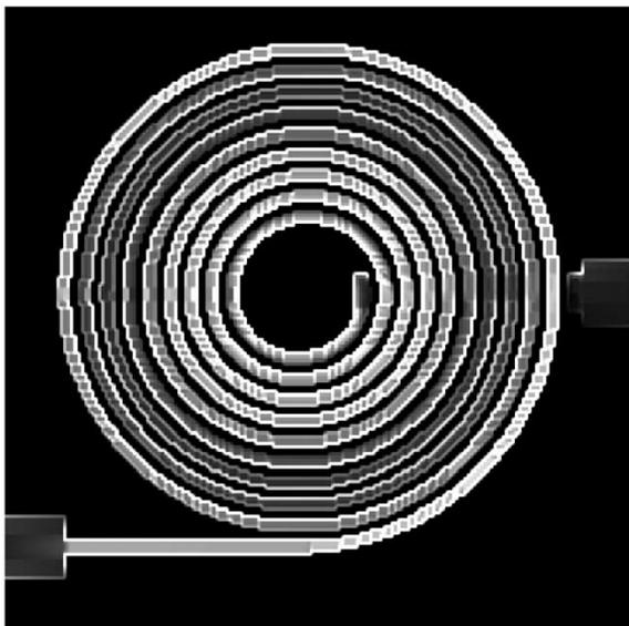
Fig. 6. Large spiral inductor on silicon shows how the edge effect current switches back and forth between sides as it flows around the spiral, illustrating the critical importance of including the edge effect when analyzing loss.
