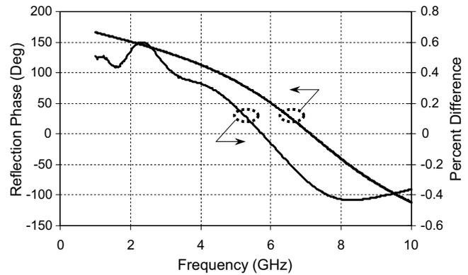
Fig. 5. Reflection phase results for both curved, shorted stubs in Fig. 4, are visually identical. Percent difference is under 0.6% at all frequencies.
