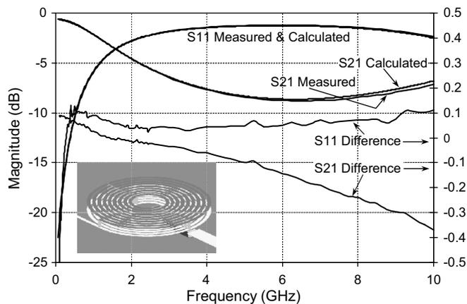
Fig. 7. Measured versus calculated for the spiral inductor on GaAs. The difference between the two is plotted on the right-hand-side axis.
