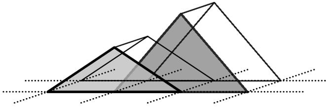
Fig. 1. Each rooftop basis function covers two cells. Two rooftops can be merged together, with appropriate weighting, to yield a larger rooftop, covering three cells. Vertical dimension indicates current density.
