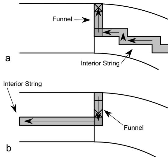
Fig. 3. (a) String on the interior of a conformal subsection allows current to flow longitudinally to the peak edge (center). From here, the current flows in a “funnel” string to the mutual meeting point indicated by the “X.” (b) In the adjacent conformal subsection, a string draws current from the mutual meeting point along its own funnel string.
