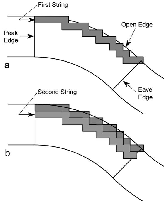
Fig. 2. Conformal meshing considers a section starting with the “peak edge” and ending with the “eave edge.” One outside edge is considered the “open edge,” where the high edge current flows. (a) The path for the first string goes along this edge. (b) A second string is added.
