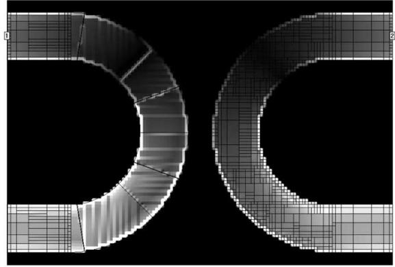
Fig. 4. With normal subsectioning on the right, we can see the dramatic reduction in subsection count provided by conformal subsectioning on the left. The general nature of both current distributions is the same, especially in regard to the edge effect.
