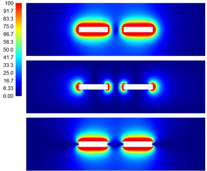
Fig. 3. Even-mode electric field of coupled stripline. Fields are taken in the transverse plane at an open end with 1 V applied between both lines and ground. The scale on the left is in volts per meter. The top image is the total electric field, the middle image is the magnitude of the horizontal component. The bottom image is the magnitude of the vertical component (from [10]).
