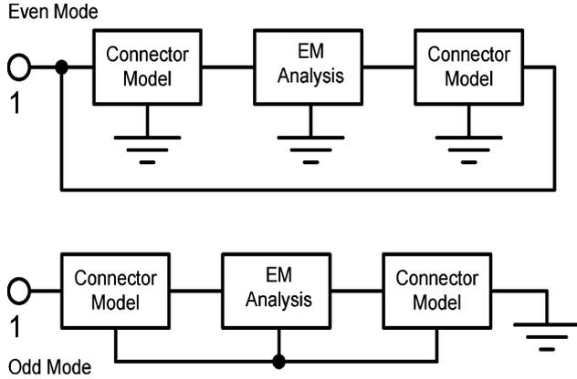
Fig. 2. Schematics for converting a symmetric two-port (EM analysis) into two one-ports yielding the even and odd modes. It is critical that the ground terminals are explicit and tied together and not connected to global ground for the odd mode.
