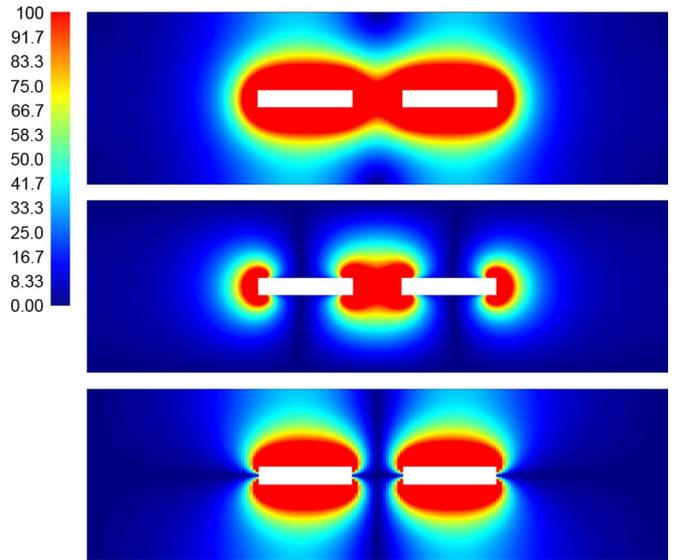
Fig. 4. Odd-mode electric field of coupled stripline. One volt is applied between the two lines. All other information is the same as Fig. 2. Fields are stronger for the odd mode because the odd-mode impedance is lower, resulting in higher current, from [10].
