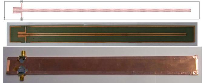
Fig. 1. RA resonator: (top) layout in Sonnet, (middle) fabricated resonator, and (bottom) completed resonator. The resonators are 10 in long. The input/output coupled region is 0.5 in long.
