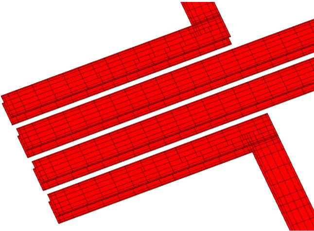
Fig. 6. Fine meshing is required in the EM analysis. The minimum subsection size (i.e., the cell size) used here is  $5 \times 2.5$  mil. The input coupling sections are 0.5 in long. The complete resonators (see Fig. 1) are 10 in long. Two sheets are used; the vertical vias connecting all edges not shown. Vertical dimension magnified 44 times.
