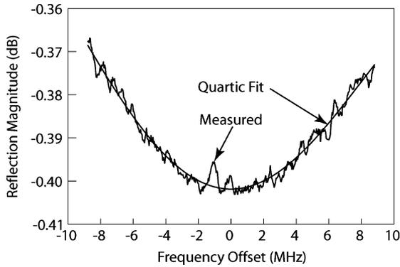
Fig. 5. Performing a least squares quartic polynomial fit on data around a resonance allows accurate extraction of the resonance even in the presence of considerable noise. This is the seventh even-mode resonance centered at 2046.172 MHz.
