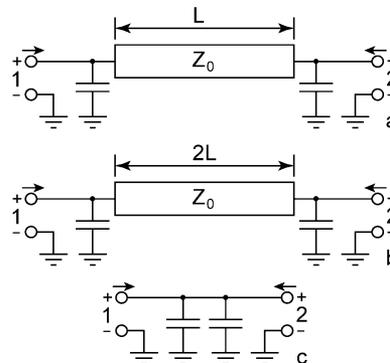
Fig. 2. Circuit theory model for the  $L$  and  $2L$ -length through of the double-delay calibration shows ports as a pure shunt admittance. After manipulating the cascading matrices, the double port discontinuity (c) remains.
